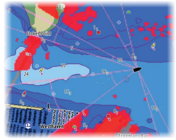
Radar overlay on a chart
